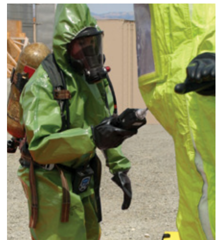
Workers can easily measure VOCs and wirelessly transmit readings up to two miles/3 km away.
